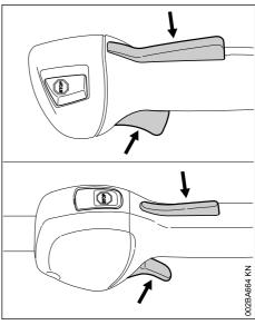
Press down the throttle trigger lockout and open the throttle – the choke knob moves to the run position I. After a cold start, warm up the engine by opening the throttle several times.
