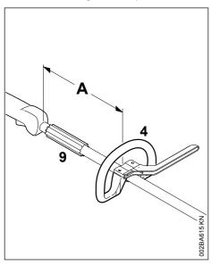
The loop handle can be adjusted to suit the height and reach of the operator and the application by changing distance (A).
