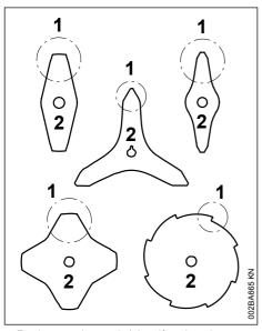
Resharpen the teeth (1) uniformly – do not alter the contour of the parent blade (2) in any way.
